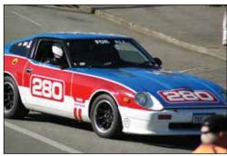
Two seater coupé, fitted with half cage, race seat and 6 point harness. Very fresh 2.8+L motor with triple 45mm Webers and MSD ignition. 4.1:1 LSD Differential with CV's.
