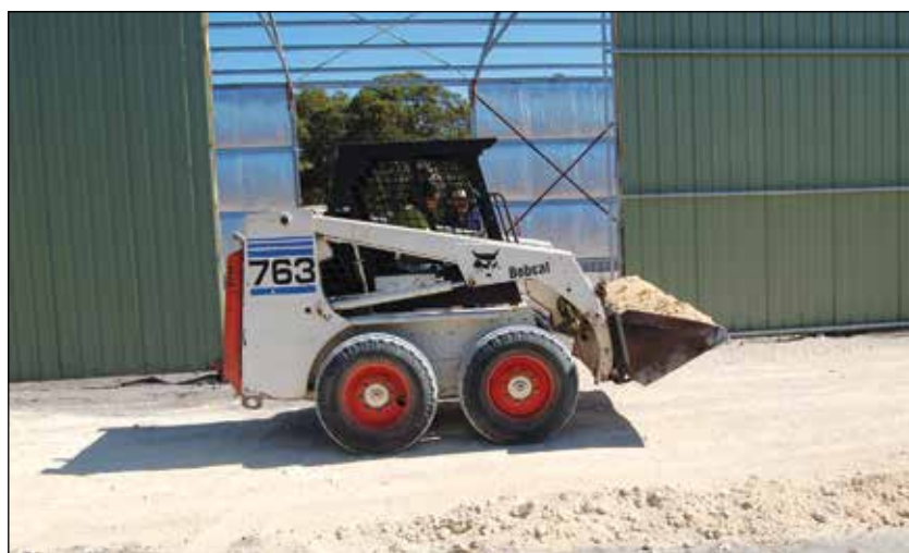
Lindsay in the trusty Bobcat thunders by with a scoop of limestone for the shed pad apron.
